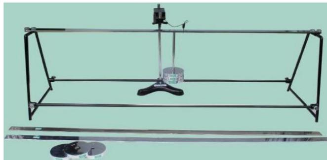
Fig. 2: Experimental setup for Young's modulus measurement
