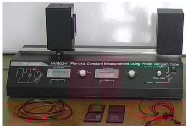
Fig. 2: Planck's constant measurement unit
