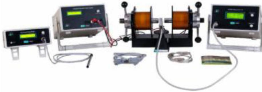
Fig. 2: Hall effect measurement unit
