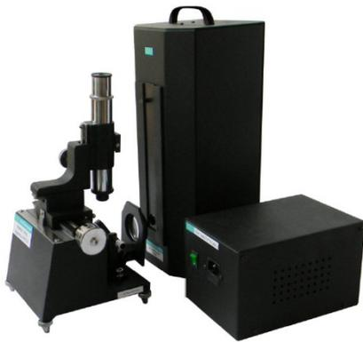
Fig. 3: Newton's ring experimental setup
