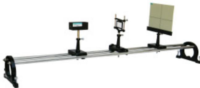
Fig. 2: Diffraction grating experimental setup
