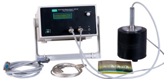
Fig. 2: Band gap measurement unit
